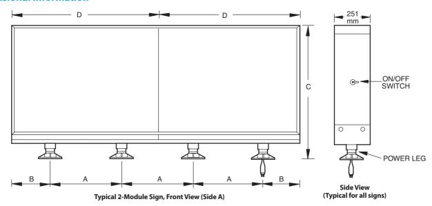
**Sign Power Leg Orientation** When facing side A, the power entry is on the right. Orders should always specify the message orientation.
