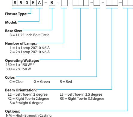
A = Standby Lamp (Series Circuit): Energizes standby lamp upon failure of operating 150 W lamp.\*\*
